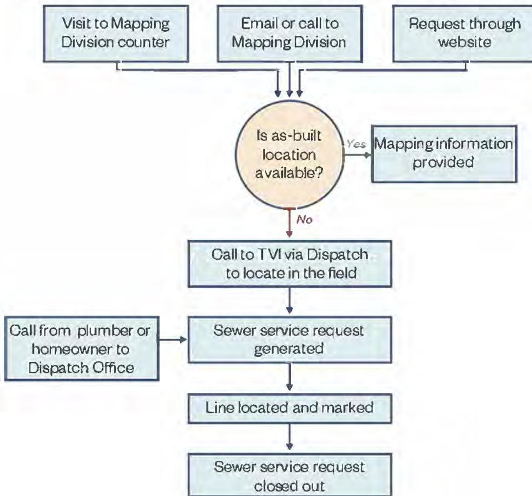
Figure 1. Sewer Lateral Location Request Flow Diagram
