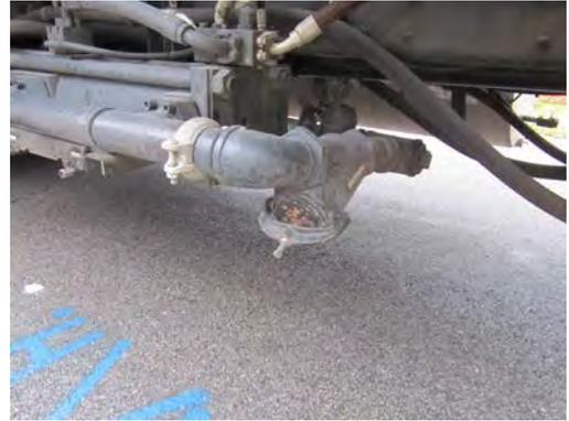
6. Check water strainer at the fill inlet to the water tanks.
