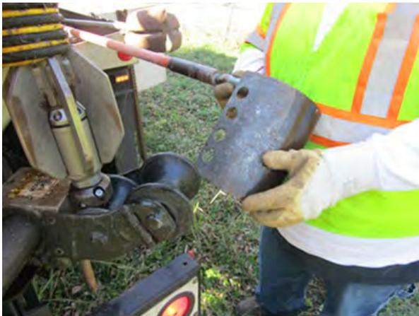
**Photo 7-1. Debris Traps and Poles Used to Set Debris Trap in Manhole Channel**
