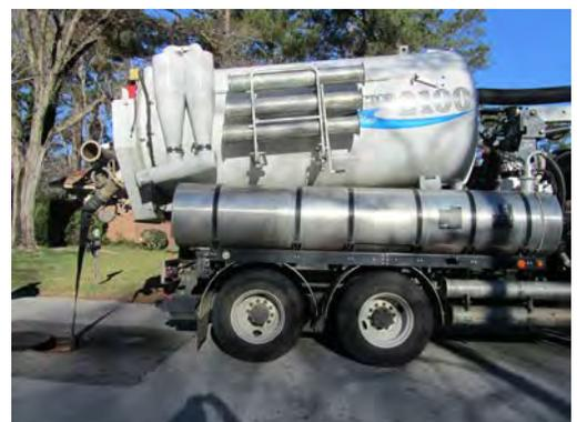
8. Open the decant valve slowly, and wait until flow stops before raising the debris body.
