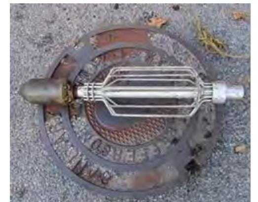
18. On the final cleaning pass, maintain a nozzle return speed of 35 to 40 feet per minute. Use the white marking on the reel speed control valve as an indicator for this rate.
