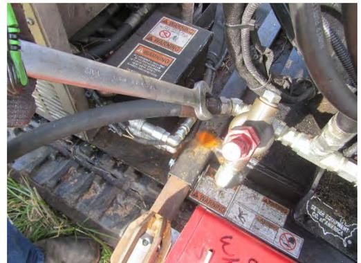
9. Select the appropriate cleaning nozzle for the job, verify that a tiger tail is on the easement machine sewer cleaning hose, and attach the nozzle to the hose.
