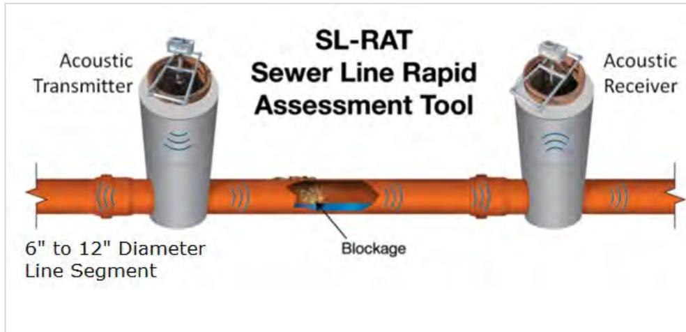
**Figure 7. SL-RAT Concept and Operational Procedure**
