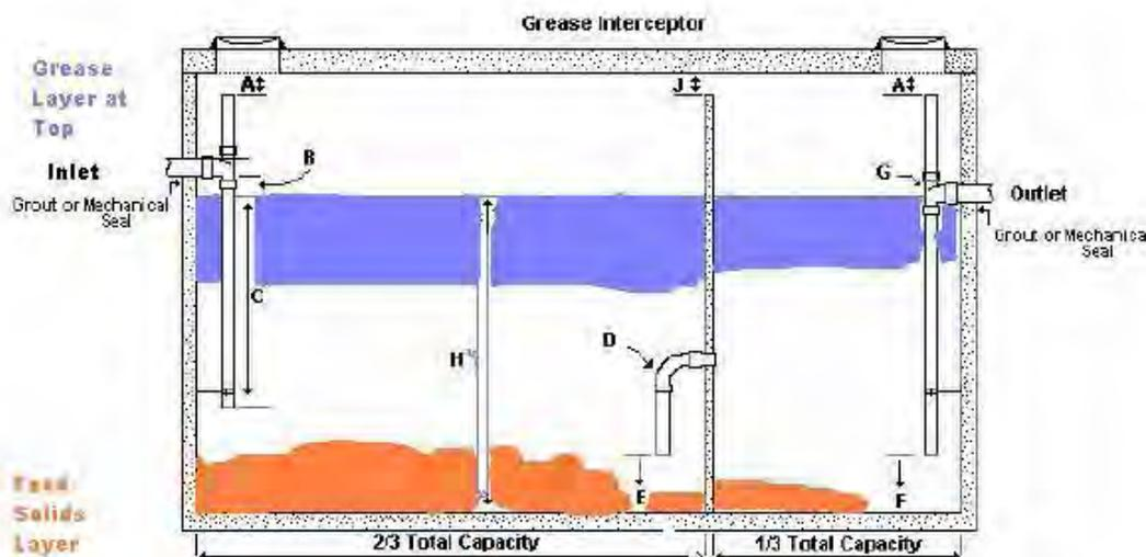
*Why a complete pump of the Grease Trap is necessary:* Both the FOG layer and the food solids layer take up capacity in the trap. The food solids layer will normally be 1x to 2x the FOG layer depth. If the FSE prepares chicken, seafood or rice, the food solids layer will be 2x to 4x the FOG layer. Thus, short-circuiting of the grease trap can occur if the full contents of the trap are not pumped.
