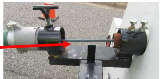
Perform tool changes at the far manhole during operations; perform heavy cutting while pulling back. Use a gaff to guide the tool and string of rod to the top of the manhole.
