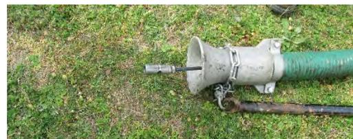
6. Verify the lower rod guide hose brace is attached to the bell end of the guide hose and has a rope attached for insertion and removal.
