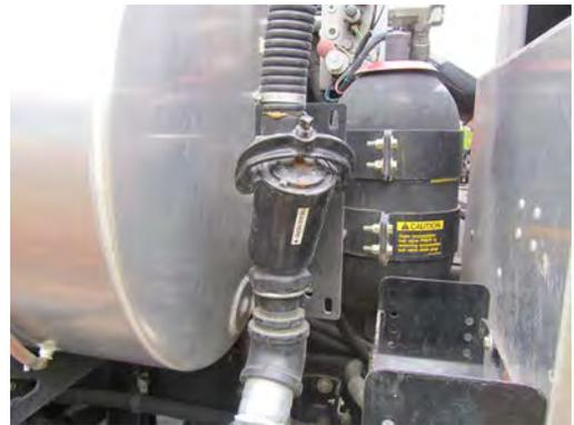
7. Using the water pump blow out valves, remove debris in the water pump. With the trunk engine set to idle and the water pump cycling at a low RPM, engage the pump and gently open and close the blow out valve. Blow out and close each valve, one at a time.
