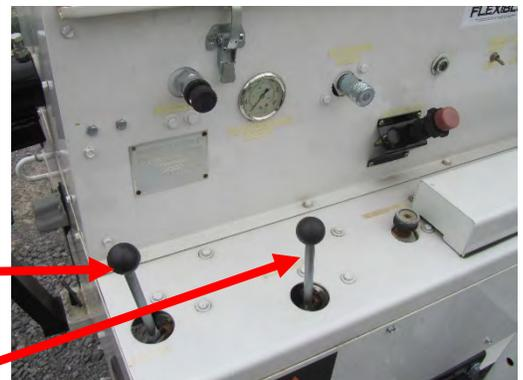
5. Rotation speed for augers (and all boring tools) is approximately 25 rpm, which is adjusted using the reel rotation control. Color rings are used as markers to set rotation speed.
