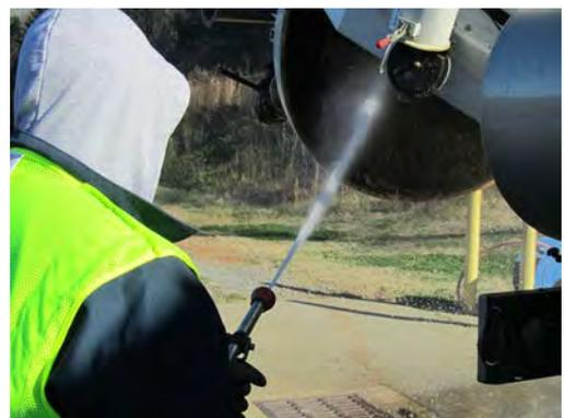
6. Lower the debris tank, clean up any material spilled on the cleaning pad.
