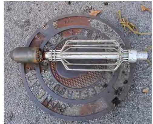
18. On the final cleaning pass, maintain a nozzle return speed of 35 to 40 feet per minute. Use the white marking on the reel speed control valve as an indicator for this rate.
