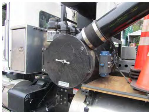
5. Close the water tank valve to the pump and check the strainer at the water pump. Remove any debris found in the strainer and replace.
