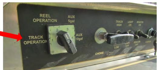
5. If moving back to the trailer, disconnect the water supply hose from the easement machine to the water supply truck reel in order to rewind the sewer cleaning hose to the truck. Assist the process by hand when the hose becomes snagged or tangled along the way.
