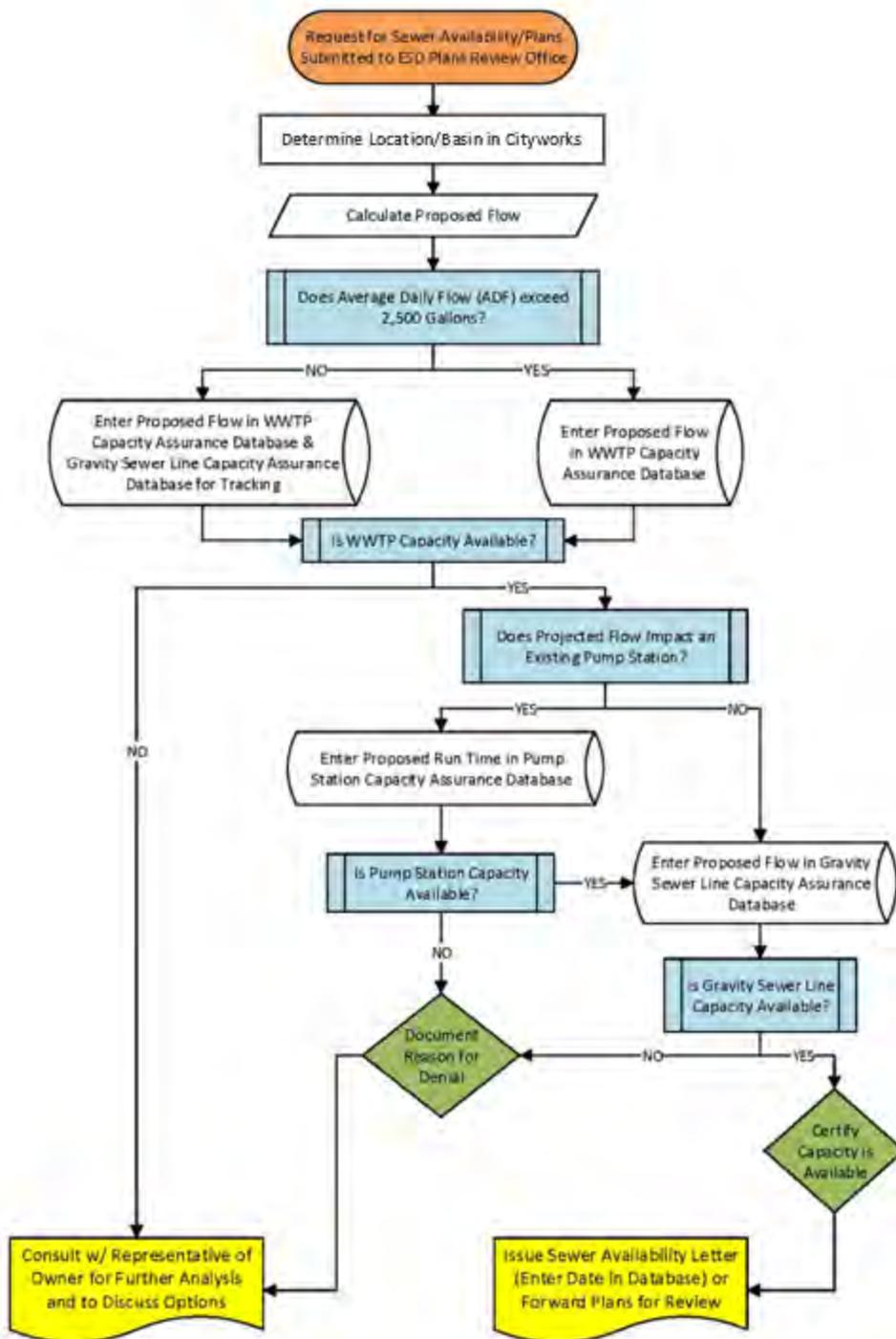
Figure 12. Permit and CAP Process Flow Diagram
