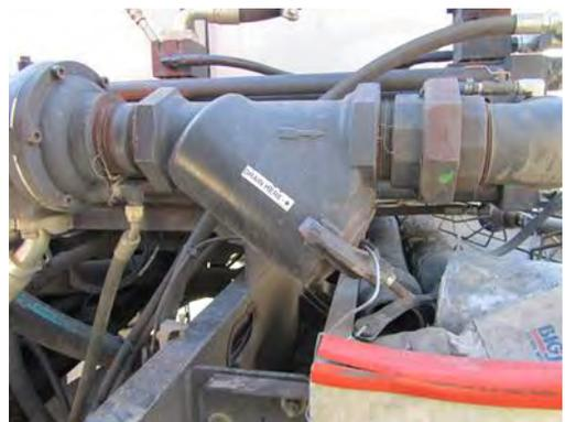
4. Using the water pump blow out valves, remove debris in the water pump. With the truck engine set to idle and the water pump cycling at a low RPM, engage the pump and gently open and close the blow out valve. Blow out and close each valve, one at a time, twice.
