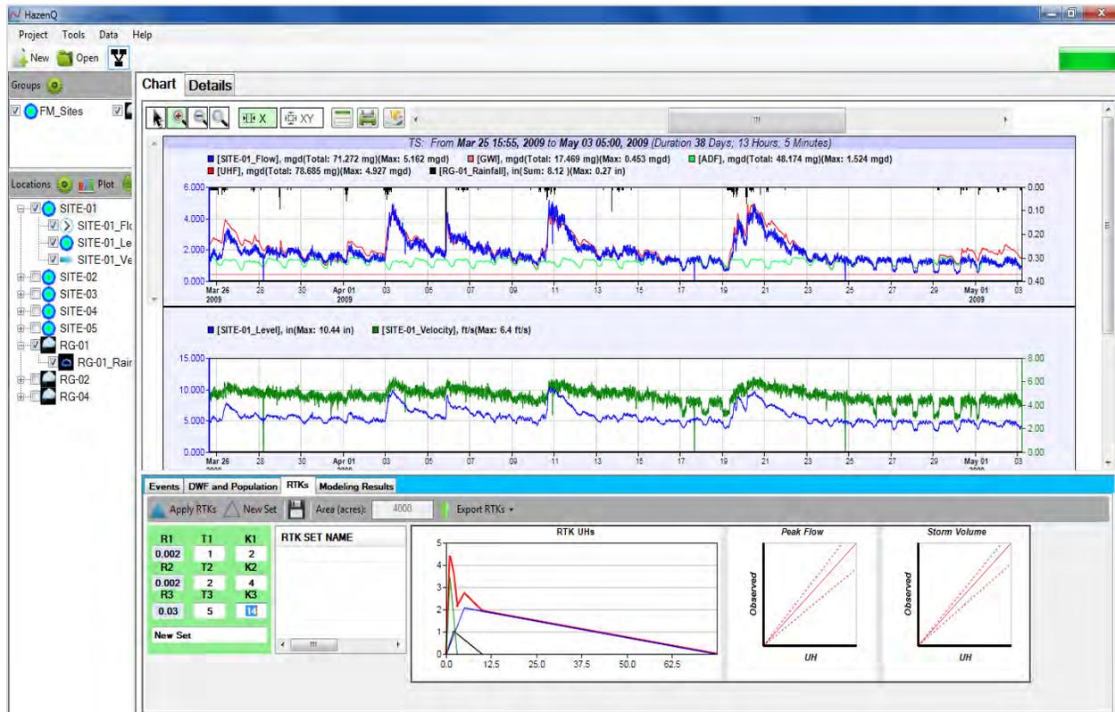
**Figure 7.RTK Generator**
