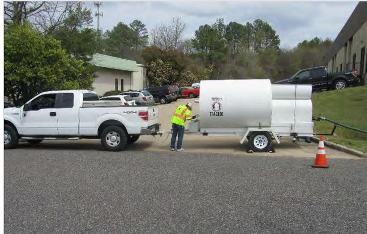
**Figure 5. Trailer Mounted Power Rodding Machine**
